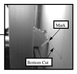
4. Move the head right to the start of the bottom cut. Make a starting mark on the front recess of the foot.
