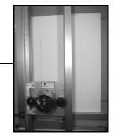
Position the knife head in the middle of the bottom cut. Make a border setting mark on the left side of the foot.
